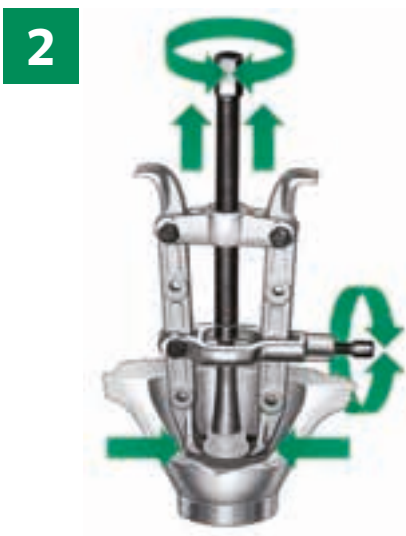
How a two-armed puller works
