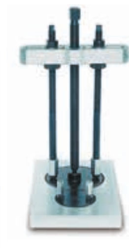
Puller in use for removing gearwheels
